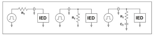
Critical lines may be either **source terminated** (left) or **load terminated** (center, right). Load terminations can be either dc (center) or ac (right). All will give similar performance so far as damping undesired ringing and overshoot, though they have different characteristics in other ways:
