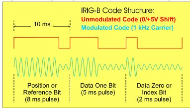
The unmodulated IRIG-B code can deliver accuracy limited only by the slew rate of the digital signal, much better than one microsecond and, with care, in the range of a few nanoseconds. Unmodulated IRIG-B is normally distributed at a level of 5 volts (compatible with TTL or CMOS inputs). While some IEDs couple the IRIG-B signal directly to a logic gate,
