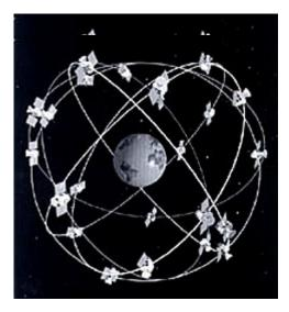
data on the satellite's precise location and time. The satellites are equipped with atomic clocks that are precise to within a billionth of a second. The control segment continually monitors performance of the satellites and adjusts their internal clocks as required to maintain accuracy.
