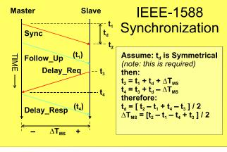
IEEE Standard 1588 provides for both software-only and hardware-aided implementations. Software-only PTP implementations have demonstrated timing accuracy of 10 to 100 us (similar to NTP in a small local area network); in contrast, hardware-assisted PTP implementations have demonstrated accuracy of 20 to 100 ns. **Note that to achieve timing accuracy better than 10 us, all devices must run hardware-assisted PTP implementations.**
